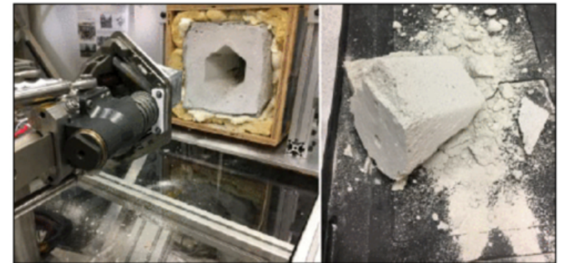
(b) Sample acquisition from a 5.2 MPa simulant block during penetration test.
